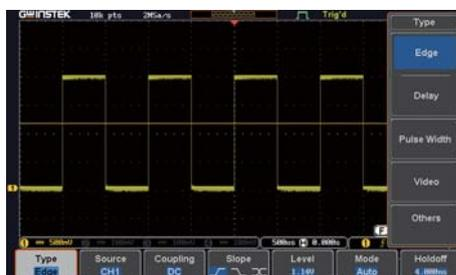
The GDS-1000B series oscilloscope is equipped with diversified trigger functions, including Edge Trigger, Delay Trigger, Pulse Width Trigger, and Video Trigger. Engineers, based upon different waveform measurements, can select different trigger functions to lock waveforms in order to identify the root cause of the complicated circuit designs to save development time and to accomplish tasks.
