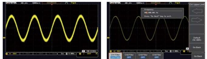
In electric circuit tests, engineers are often troubled by noise interference while measuring signals. The GDS-1000B series oscilloscope provides the digital filter function option, which can be set as high pass or low pass filter. The filter frequency can be adjusted according to the requirements. The filter parameters of each channel can also be set. The tracking on function can be used to set same filter frequency for all channels.
