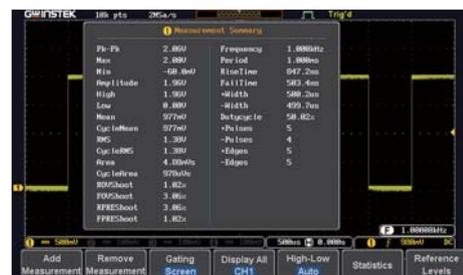
display screen. Users can also select to show all parameters if the preset eight sets are insufficient. Once the selection is made, all 36 measurement parameters will be shown on the center of the display screen. This is a very convenient measurement tool for students writing dissertations or engineers writing reports.
